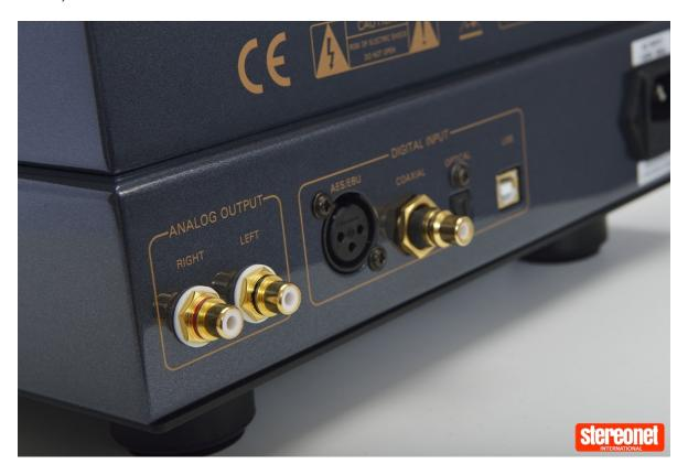
Four digital inputs are offered – USB, S/PDIF RCA coaxial, AES/EBU XLR, and S/PDIF TOSLINK optical. The analogue output is fixed and uses RCA sockets. The front panel display
