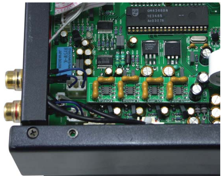
ProLogue Eight with Super I/V Op Amp board installed
