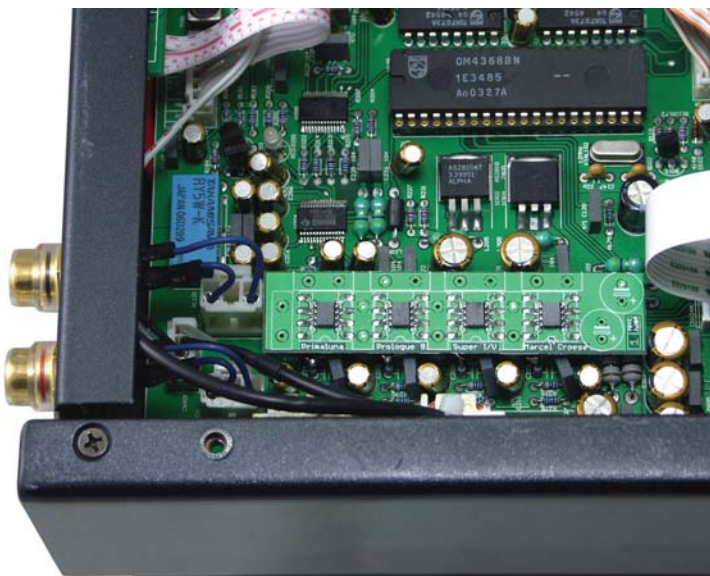
ProLogue Eight with Super I/V Basic Op Amp board installed
